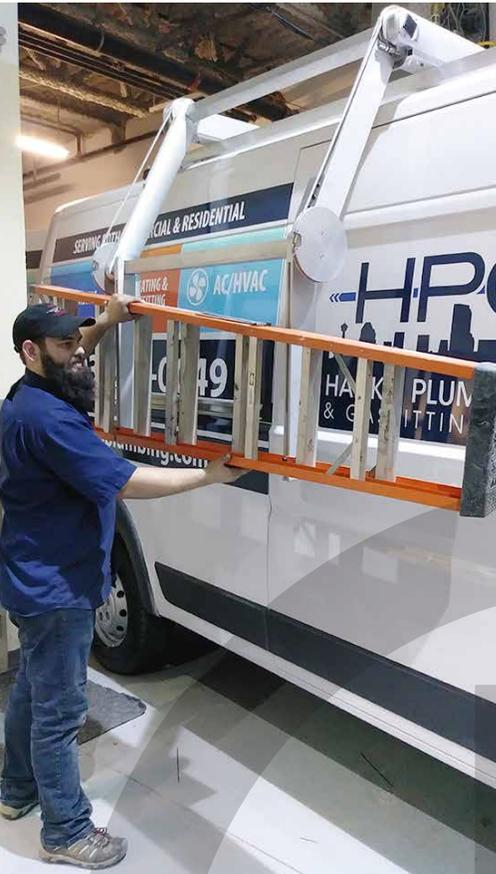
The **RazerLift** keeps the worker's arms in the green zone, providing excellent ergonomics and reducing the likelihood of injuries associated with exertion and overexertion.
